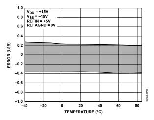
Figure 10. AD5531 Typical DNL Error vs. Temperature
