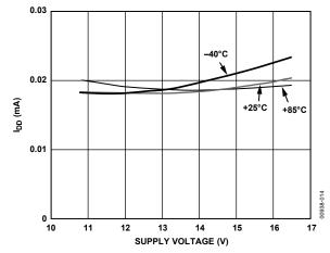
Figure 14. IDD in Power-Down vs. Supply
