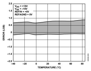
Figure 9. AD5531 Typical INL Error vs. Temperature
