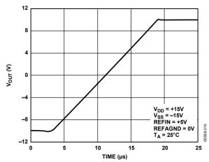
Figure 15. Settling Time
