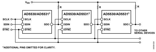
Figure 28. Daisy-Chaining Multiple AD5530/AD5531s
