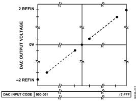
Figure 22. Output Voltage vs. DAC Input Codes (Hex)
