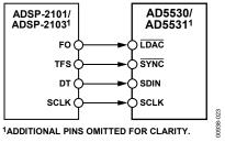
Figure 23. AD5530/AD5531 to ADSP-21xx Interface
