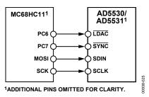
Figure 25. AD5530/AD5531 to MC68HC11 Interface
