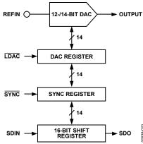
Figure 20. Simplified Serial Interface
