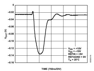
Figure 16. Typical Digital-to-Analog Glitch Impulse
