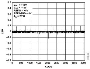
Figure 6. AD5530 Typical DNL Plot
