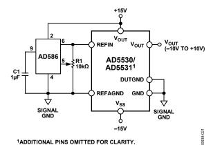
Figure 21. Bipolar  $\pm 10\, V$  Operation
