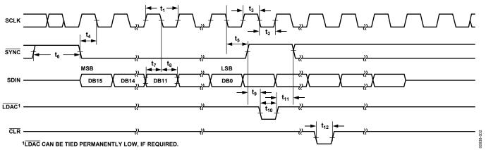
Figure 2. Timing Diagram for Standalone Mode
