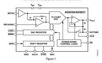
The DAC output is buffered by a gain of 2 amplifier and referenced to the potential at DUTGND.  $\overline{\text{LDAC}}$  can be used to update the output of the DAC asynchronously. A power-down  $\overline{\text{(PD)}}$  pin allows the DAC to be put into a low power state, and a  $\overline{\text{CLR}}$  pin allows the output to be cleared to a user-defined voltage, the potential at DUTGND.
