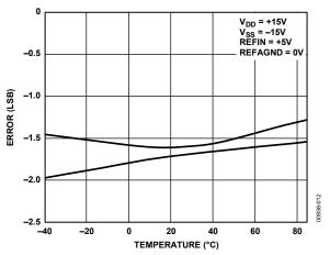
Figure 12. Typical Full-Scale and Offset Error vs. Temperature
