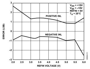
Figure 11. AD5531 Typical INL Error vs. Reference Voltage
