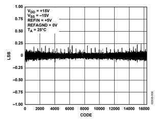
Figure 8. AD5531 Typical DNL Plot
