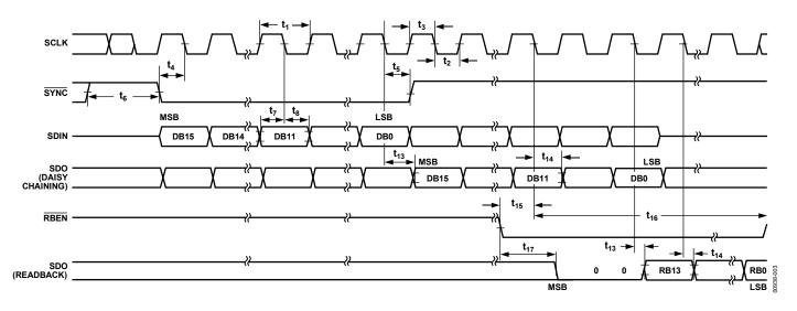
Figure 3. Timing Diagram for Daisy-Chaining and Readback Mode
