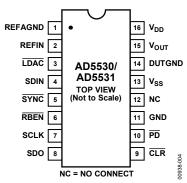
Figure 4. Pin Configuration
