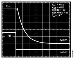
Figure 17. Typical Power-Down Time
